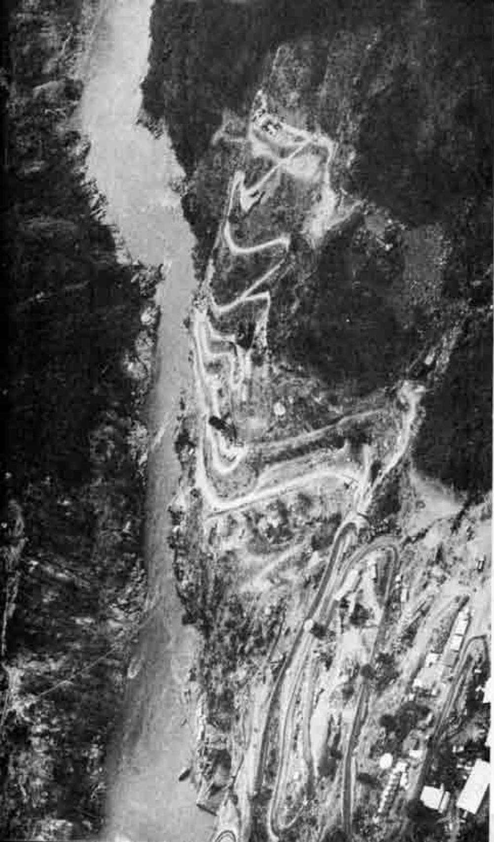
The Cabora Bassa dam site seen from the air. On the side of the cliff engineers have blasted out a hairpin bend road which is the only means of access to the site of the dam.
